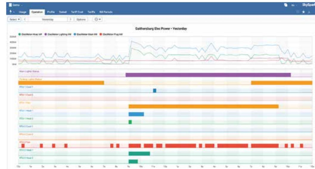
Figure 3: Operation Chart – Energy Consumption of Equipment/Systems
